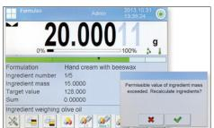
Convenient recipe-weighing: complete recipes with all recipe ingredients and associated target values, names, tolerances, tare weights etc. can be stored. If there is an excess amount of one recipe ingredient the practical back calculation function automatically calculates the new target weights of the other ingredients
