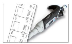
Intuitive pipette calibration in accordance with ISO 8655: The user is guided through the pipette calibration procedure step by step, in accordance with the requirements of the norm. This helps to ensure that the pipetting volumes are correct and minimises the risks in daily pipetting work
