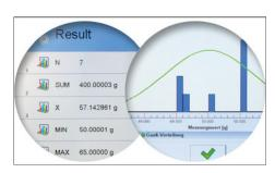
**Statistical function** for statistical analysis of series of measurements. Graphic display of measurements can be used by the operator to check and evaluate the results
